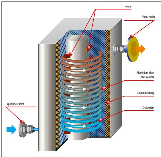
Operating diagram of dry type vaporizer FAS 2000
