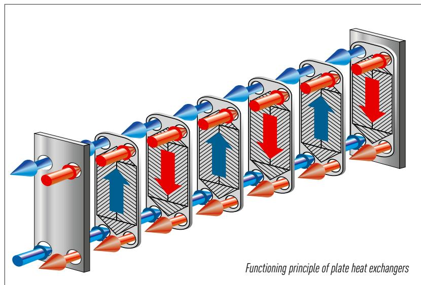
*Functioning principle of plate heat exchangers*
