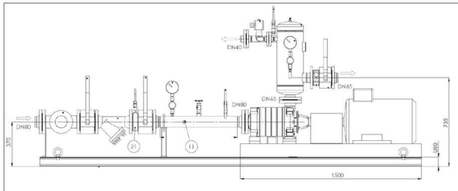
Dimensional drawing of complete suction pump unit 93 2487
