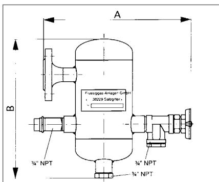
**Fine-mesh filter PN 25 for stationary systems**
