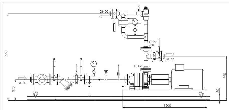
Dimensional drawing of complete suction pump unit 93 3098
