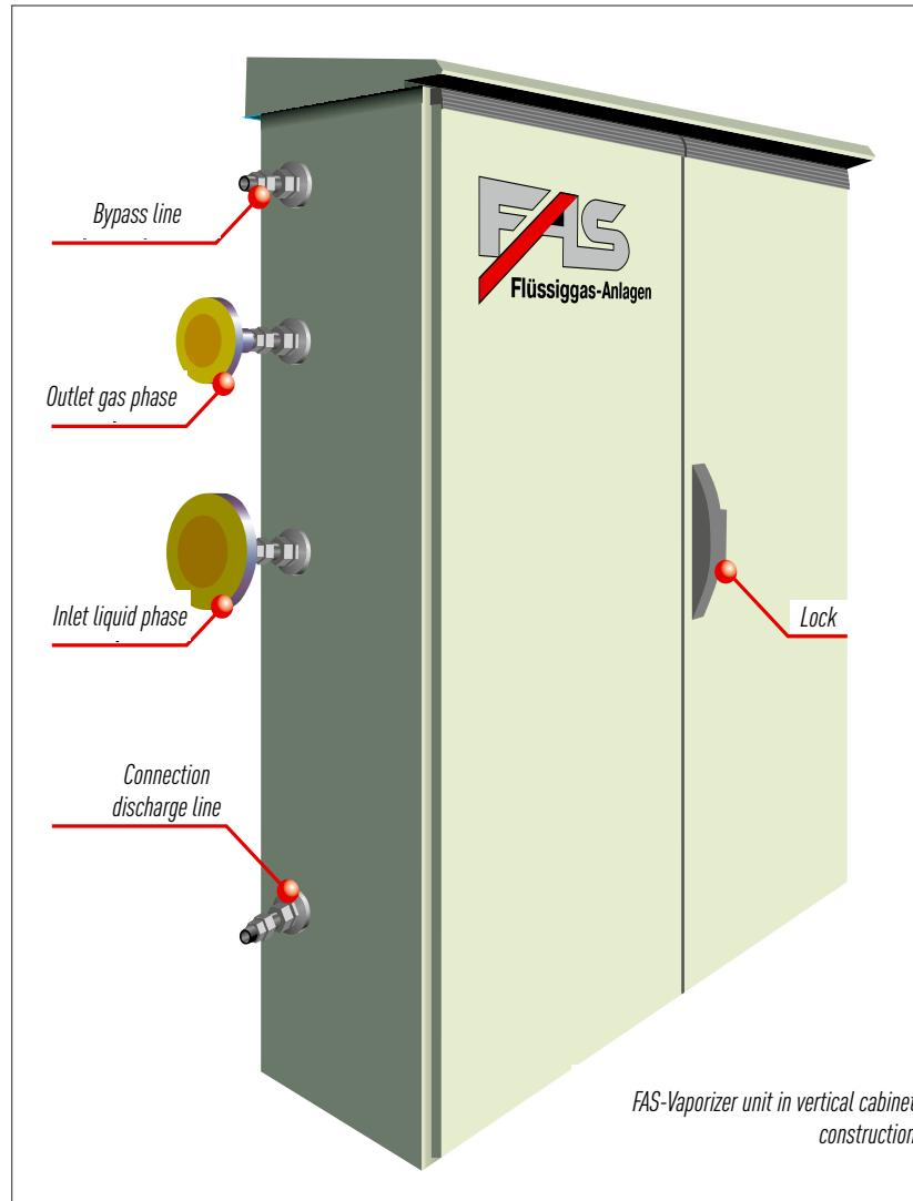
Vaporizers FAS 2000 are so called „Dry typee vaporizers“ with indirect heating. An aluminium core with high heat conductivity is used as the heat transfer medium. This ensures short warm-up and reaction time.
