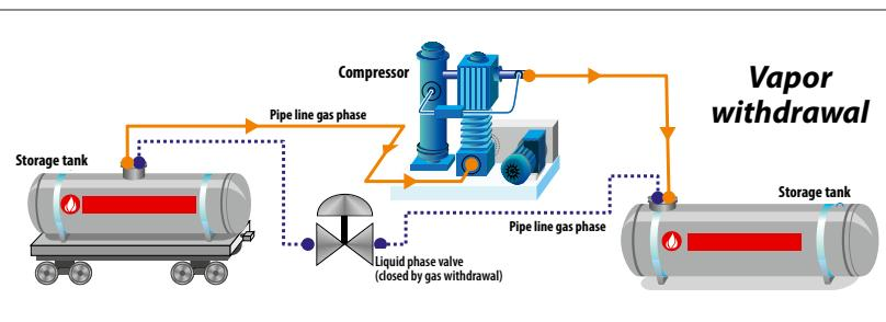
Single stage compressors (gas compression proportion less than 5:1) are normally used to transfer propane/butane from rail tankers and tank ships. Two staged compressors are used for a gas compression proportion greater than 5:1. Compressors with water coolers are used for great differential pressures and high temperatures.
