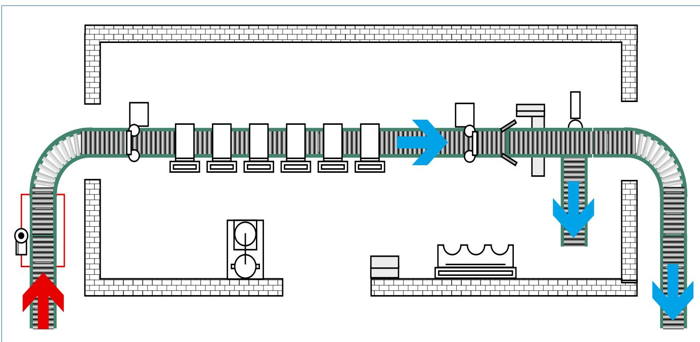
**Complete LPG cylinder refueling station in "CAROUSEL DRIVEN CONVEYOR" version**
